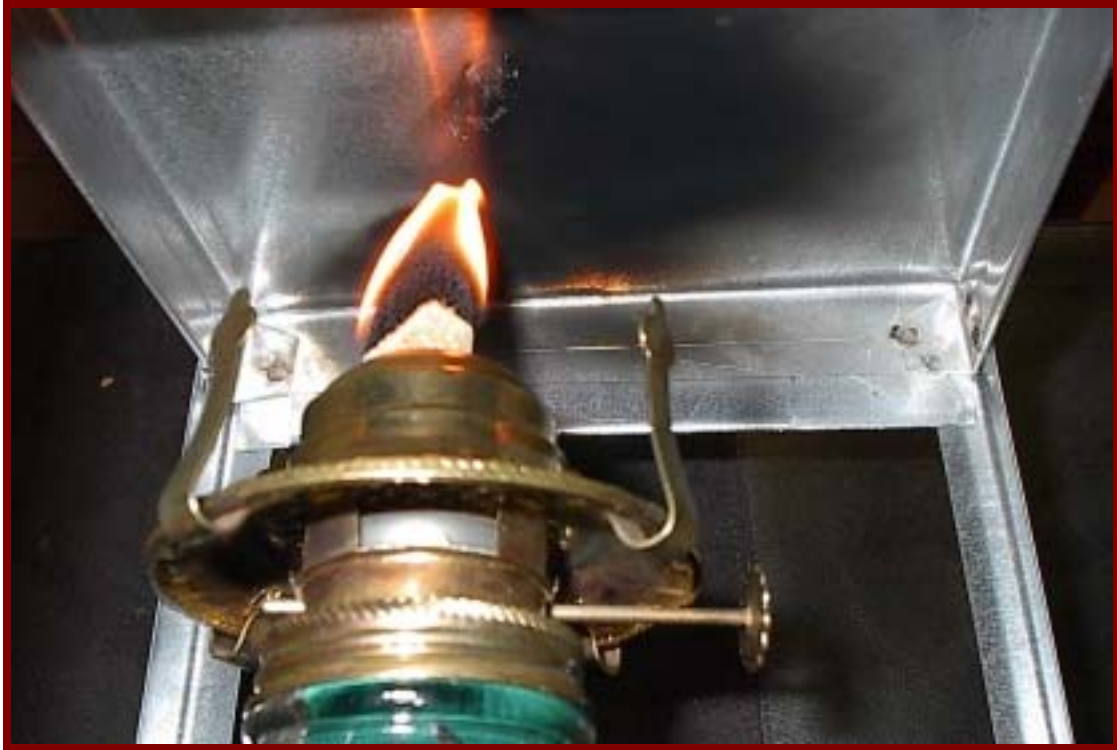
My oil lamp filled with ghee (clarified butter) and almond butter. The burning cotton wick is creating soot on the steel.
